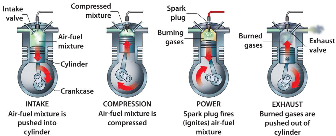
**Different Strokes** This is what happens during each stroke of a four-stroke cycle gasoline engine. *How many strokes do your legs make when you ride a bicycle?*
