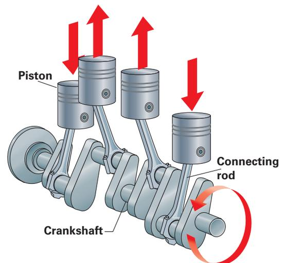
**Change in Motion** A crankshaft is a strong, heavy piece of metal that converts reciprocating motion to rotary motion. *Where have you seen something that works like a crankshaft?*
