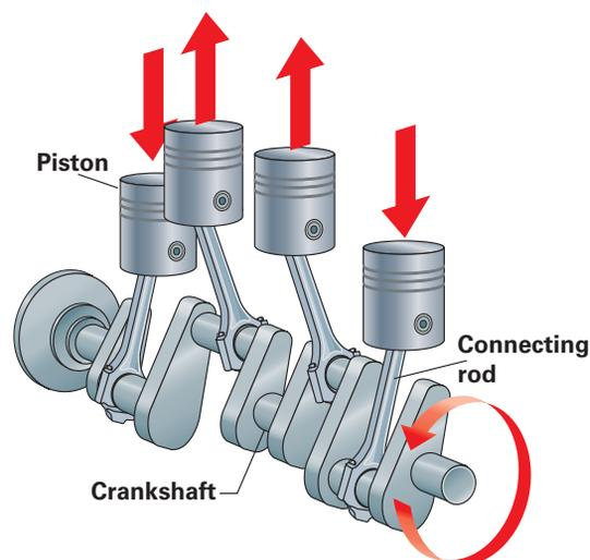
**Change in Motion** A crankshaft is a strong, heavy piece of metal that converts reciprocating motion to rotary motion. *Where have you seen something that works like a crankshaft?*
