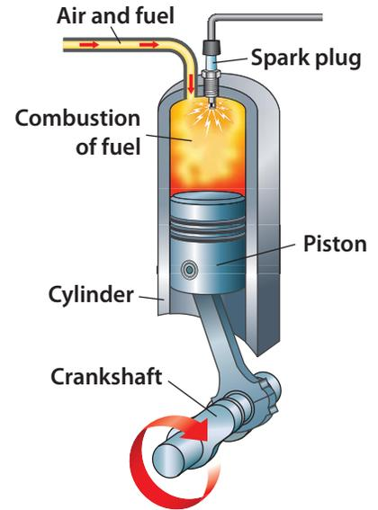
**Explosive Force** In a typical engine, fuel is ignited in the cylinder. The explosive force from the burning fuel moves the piston. *What keeps the explosive force from leaking around the outside of the piston?*
