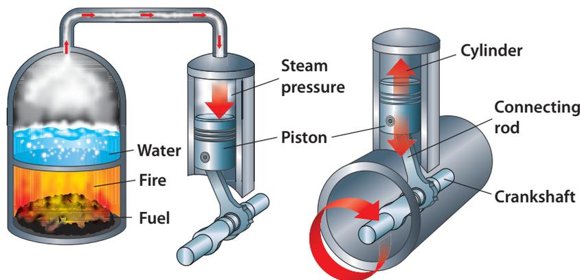
**Blowing Off Steam** Steam engines (left) produce power when steam pressure pushes on a piston similar to the one shown at the right. *What three types of fuels have been commonly used with steam engines?*
